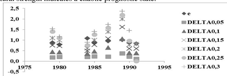
Figure 1. The mean values of capacitance (void coefficient  $e$ ),  $h u$ , and setting capacity (absolute increments of strain when the state of humidity DELTA 0,05-0,3) formations, 1978 - 1991.
